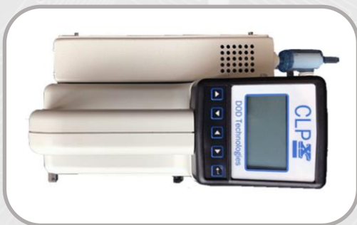
Pyrolyzer Option Detects Low Levels of NF 3
